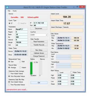
Set-up information and instant data is sent as response to "Read Parameters" command. Those are read only data. New setup must be performed in order to change those parameters.
