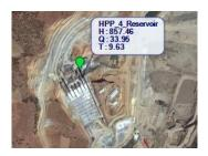
In the map window, station name, "H" water level, "Q" Flow/Capacity value, "T" water temperature are identified on station location tag. This data will be automatically updated by new values.
