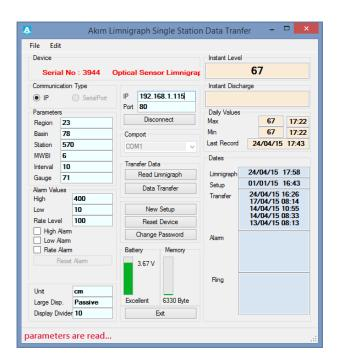
Set-up information and instant data is sent as response to "Read Limnigraph" command. Those are read only data. New set-up must be performed in order to change those parameters.
