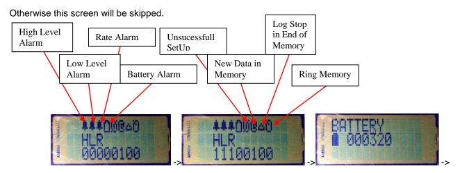
**RPRFLG** (RPRFLG Bits, the flags that enable the Alarms, from left to right, High Level Alarm, Low Level Alarm, Rate Alarm and Battery Alarms (1 = Enabled, 0 = Inactive), UNSUCCES\_SETUP, DATA\_IN\_MEM (It is "cleared" after Data Transfer; However it will be "set" again by data storage. Log Stop in End of Memory and Memory Ring flags.) Another example of RPRFLG and **Battery** Icon and level screens,
