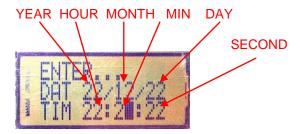
Current date and time menu is displayed. After adjusting date and time by Up and Down buttons, press Enter.
